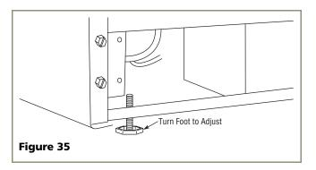
Check the levelness after each adjustment and repeat the previous steps until the unit is level. Go on to 9 Install the Unit.
